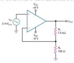
The open loop output resistance  $R_{out} = 50\Omega$ The open loop voltage gain = Avol = 75,000
