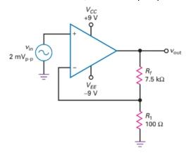
The open loop input resistance  $R_{in}=3\mathrm{M}\Omega$ The common mode input resistance  $R_{CM}=500\mathrm{M}\Omega$ The open loop voltage gain =  $A_{vol}=200{,}000$
